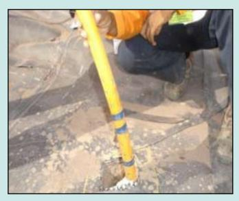
Figure 4 - Moisture sensor installation, April 2007
