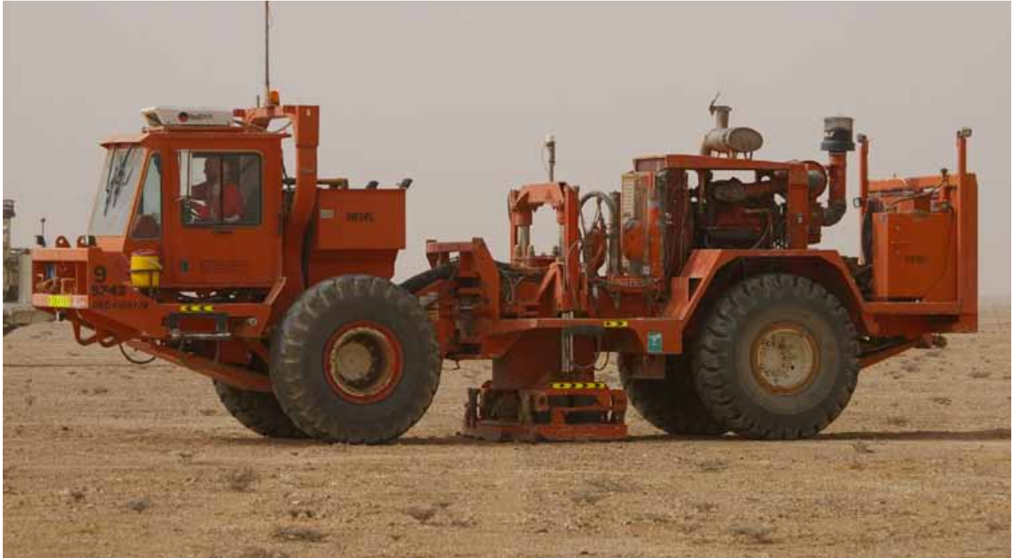
Trucks creating vibrations for recording 3D seismic data in the RSSF area. Seismic provides an image of the rock layers underground and the interpretation of this data underpins most drilling activity.
