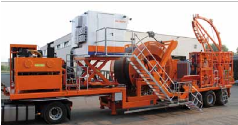
Oil Serv coiled tubing trailer
